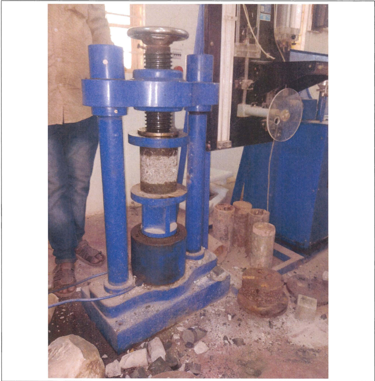
Figure 1: Compressive strength testing of the stabilized core specimen
