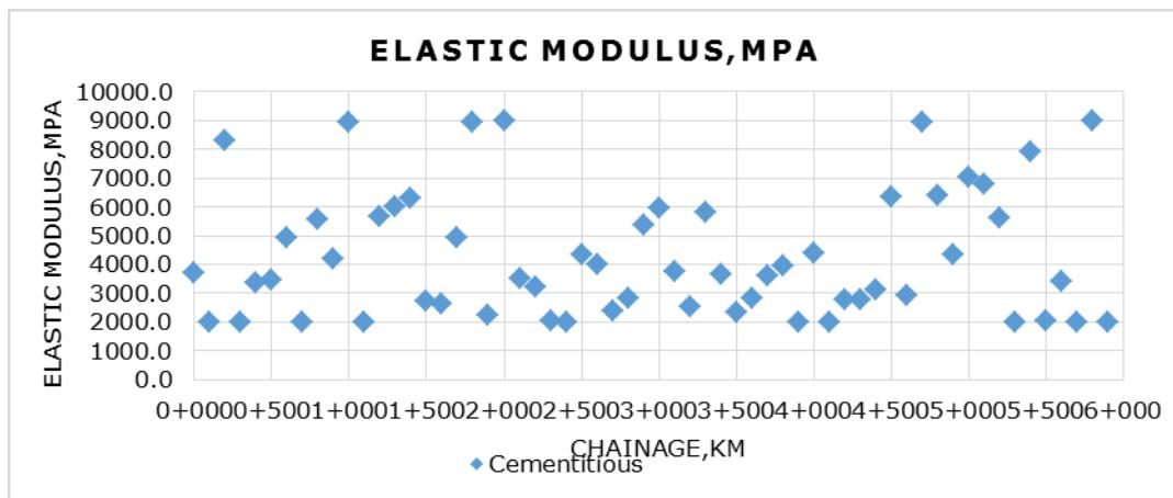
**Figure 16: Elastic Modulus of Cementitious Layer**
