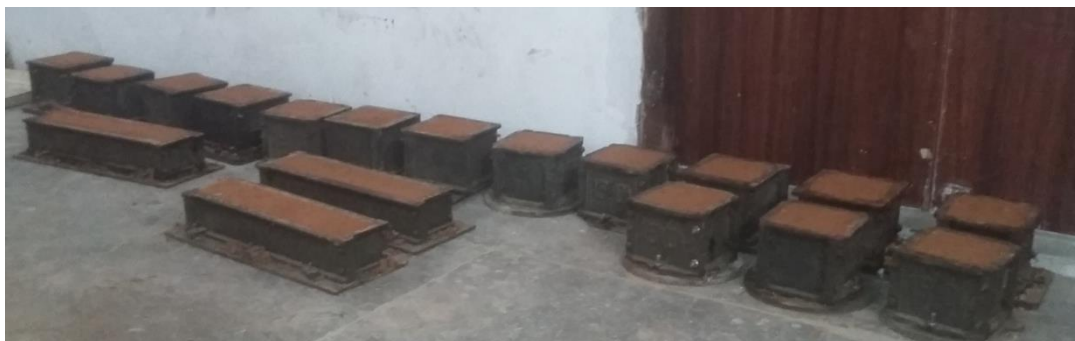
Figure 6 Compaction and preparation of UCS and Durability cubes
