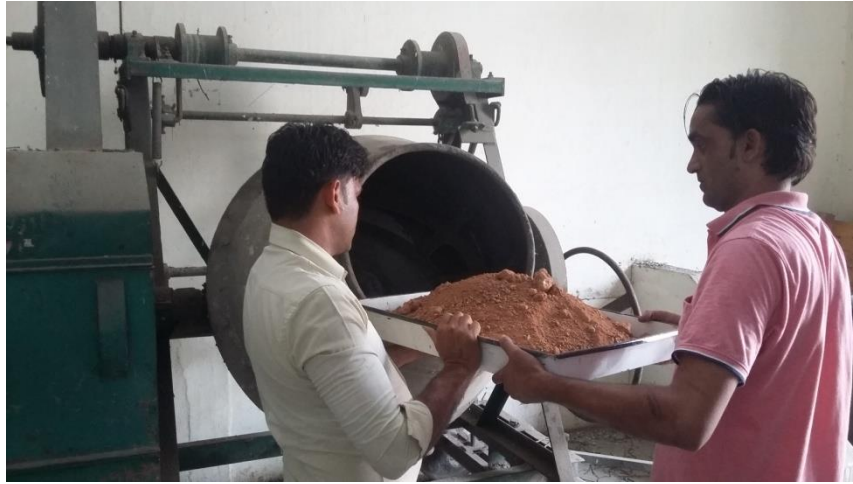
Figure 5 Mixing of stabilized soil sample
