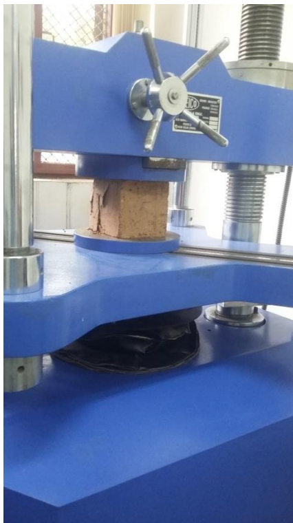
Figure 11 Residual UCS test (after durability cycles) on KP stabilized soil cubes
