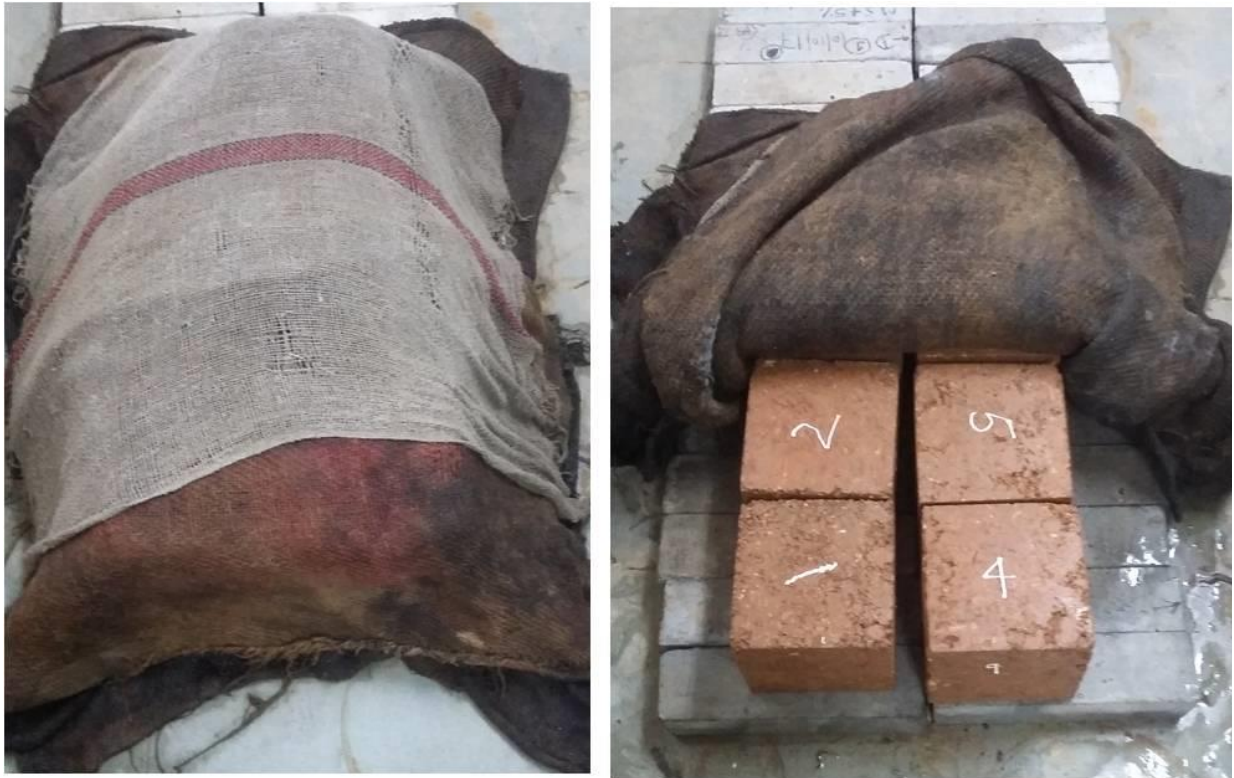
Figure 7 Curing of stabilized soil samples
