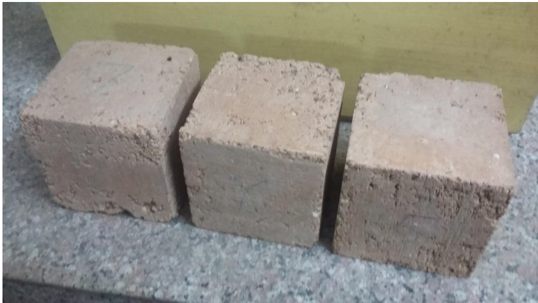
Fig. 10 Condition of stabilised soil specimen after durability test
