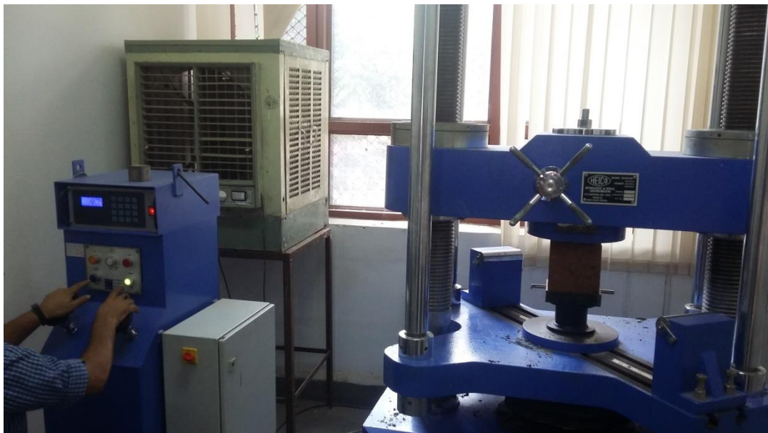
Figure 8 Unconfined compressive strength test of cubes
