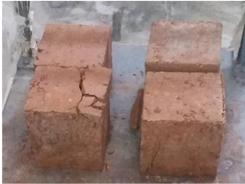
Figure 9 Failure pattern of UCS test cubes
