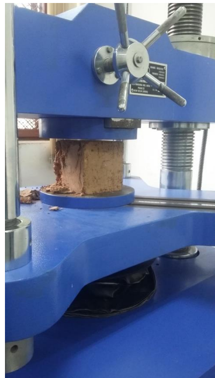
Figure 11 Residual UCS test (after durability cycles) on KP stabilized soil cubes
