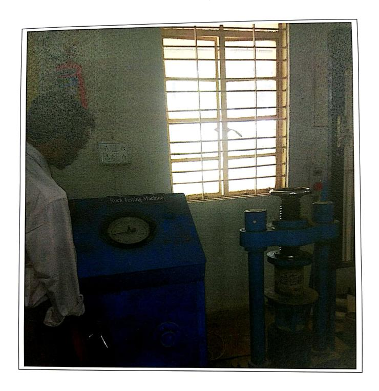
Figure 1: Compressive strength testing of the stabilized core specimen
