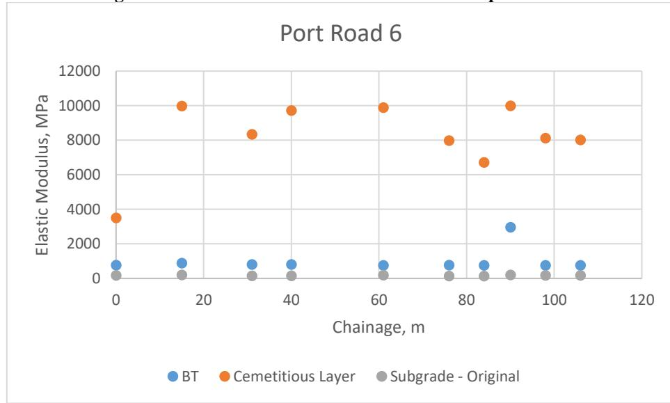
**Figure 5-12 Back-calculated E-moduli Value for port Road 6**
