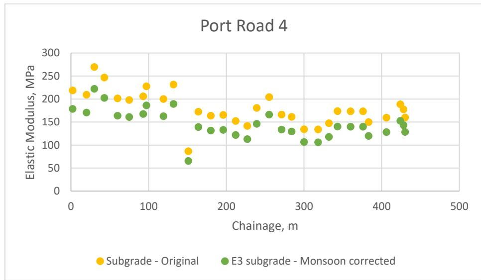
**Figure 5-22 Elastic Modulus Layer 3 Subgrade Layer Seasonal corrected at port road 4**
