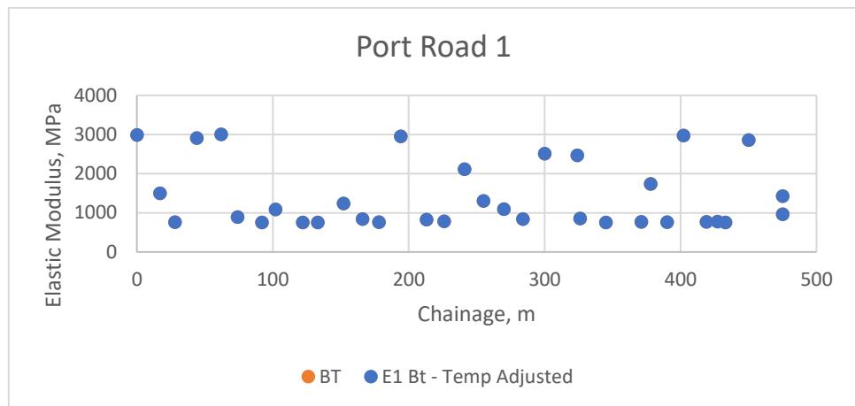
Figure 5-13 Elastic Modulus Layer 1 Temperature Adjusted @ Port Road 1
