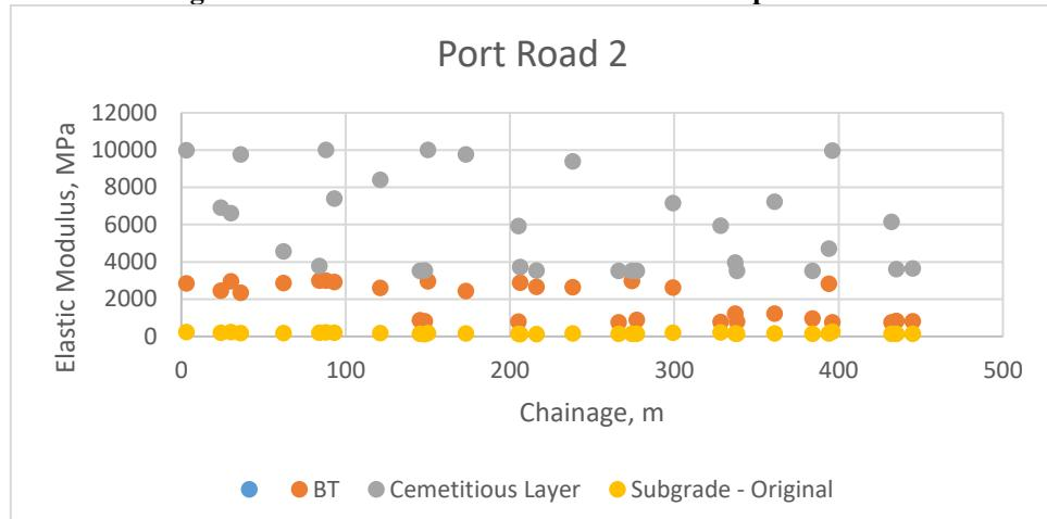
**Figure 5-8 Back-calculated E-moduli Value for port Road 2**
