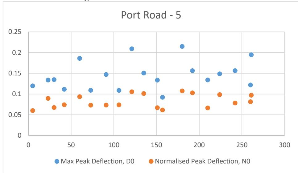
**Figure 5-5 Peak Deflection @ Port Road 5**
