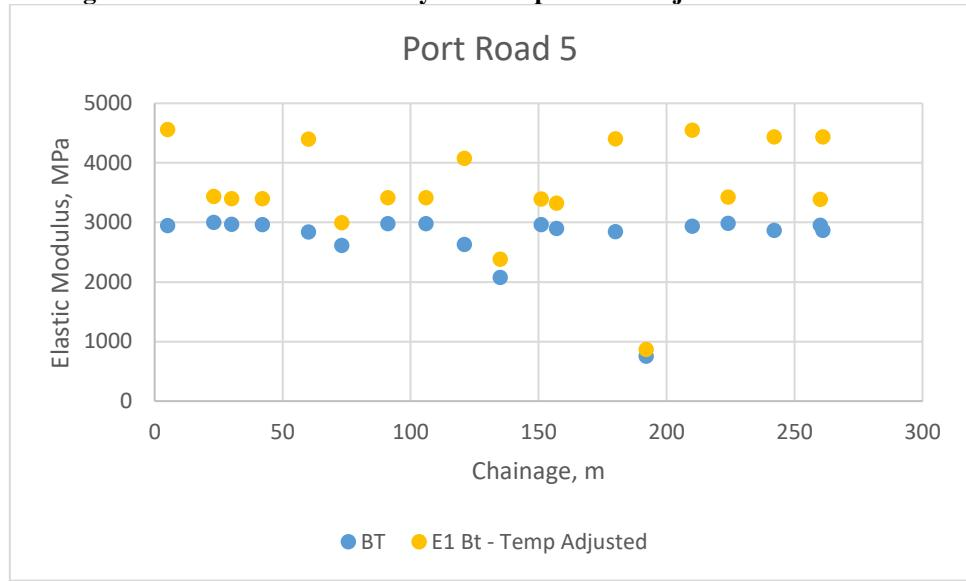
**Figure 5-17 Elastic Modulus Layer 1 Temperature Adjusted @ Port Road 5**
