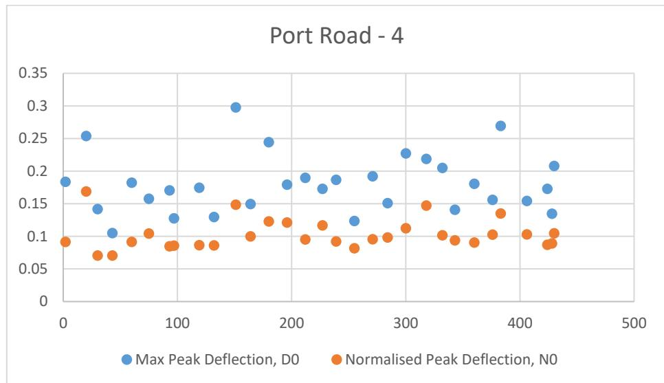
**Figure 5-4 Peak Deflection @ Port Road 4**
