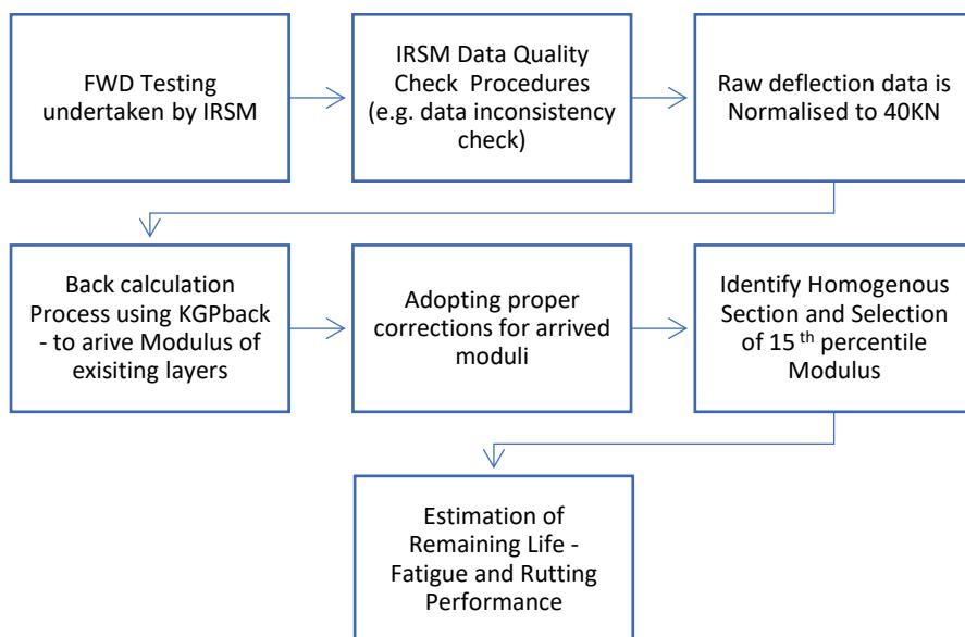
**Figure 4-1 Process Flow to determine pavement modulus values**
