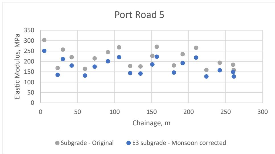
**Figure 5-23 Elastic Modulus Layer 3 Subgrade Layer Seasonal corrected at port road 5**
