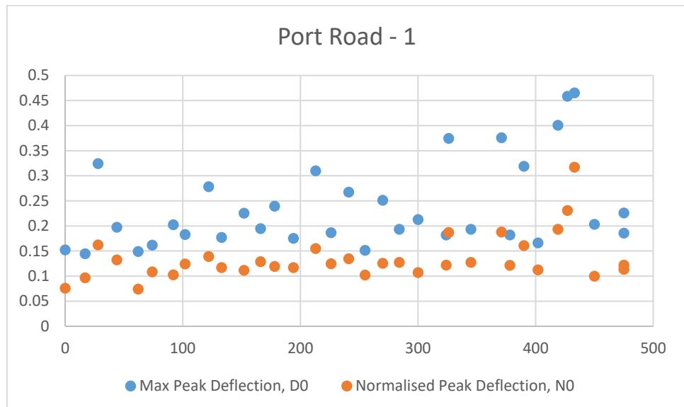
**Figure 5-1 Peak Deflection @ Port Road 1**
