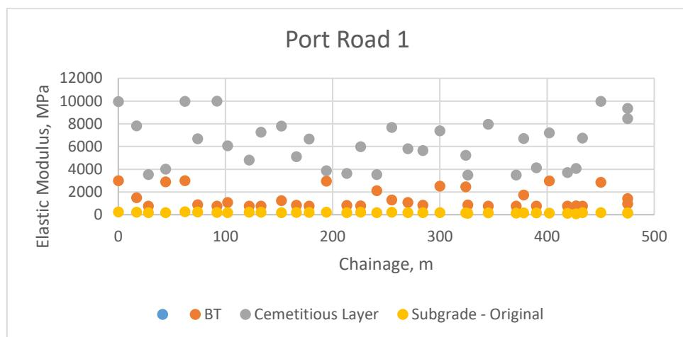
**Figure 5-7 Back-calculated E-moduli Value for port Road 1**
