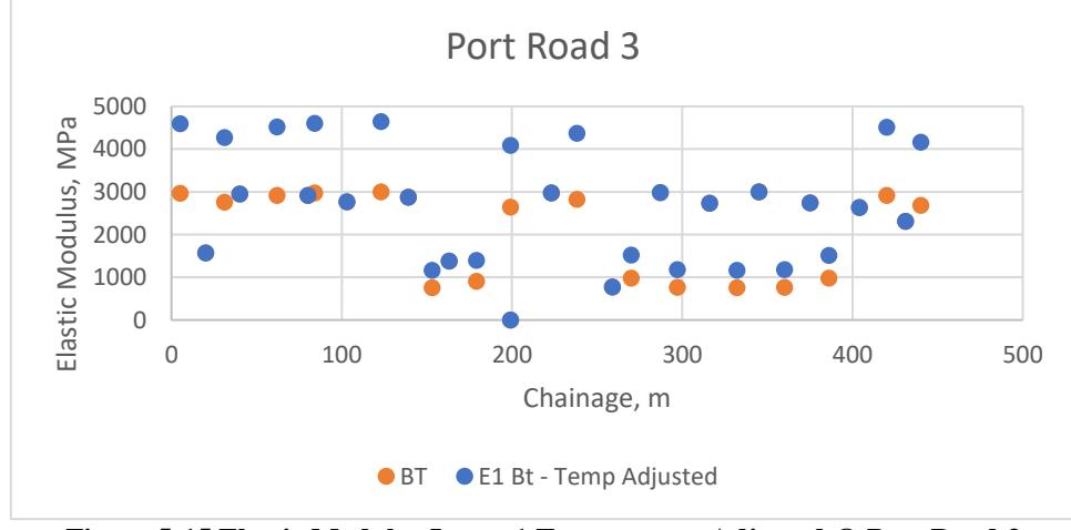
Figure 5-15 Elastic Modulus Layer 1 Temperature Adjusted @ Port Road 3
