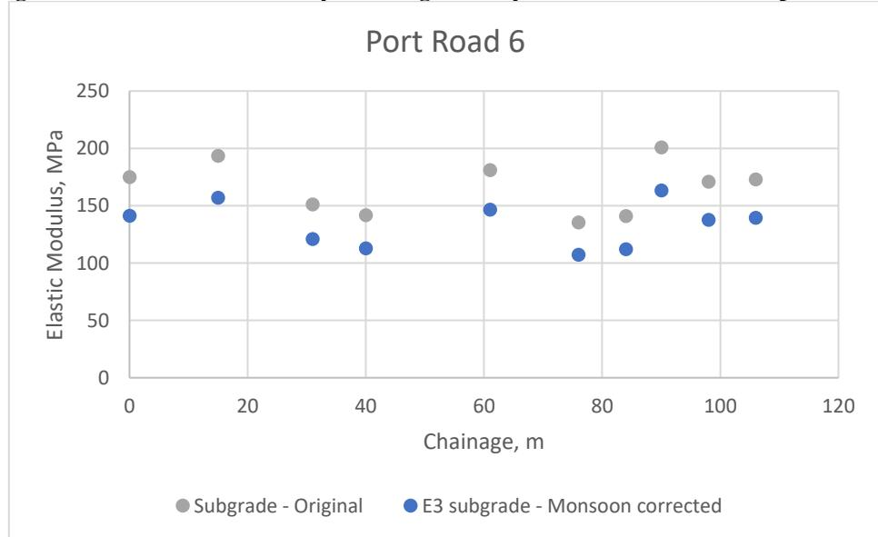
**Figure 5-24 Elastic Modulus Layer 3 Subgrade Layer Seasonal corrected at port road 6**
