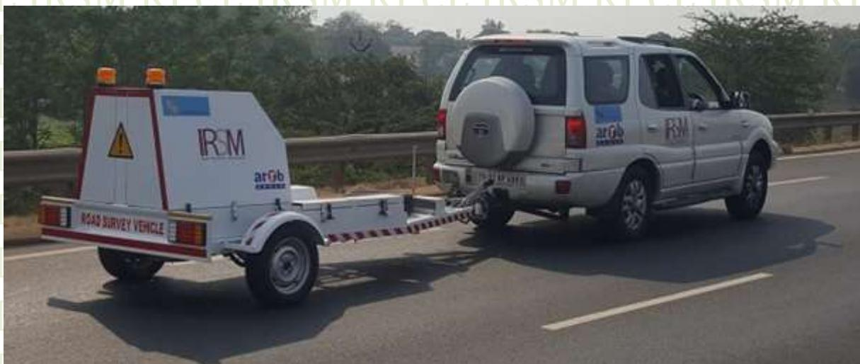
Using IRSM SWECO PRI2100 Falling Weight Deflectometer
