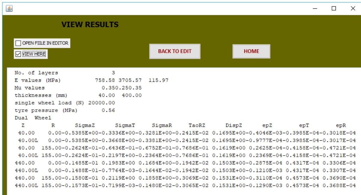
Figure 4-6 - Obtaining required strain values for checking Fatigue and Rutting performances.
