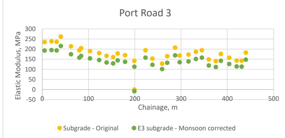
**Figure 5-21 Elastic Modulus Layer 3 Subgrade Layer Seasonal corrected at port road 3**
