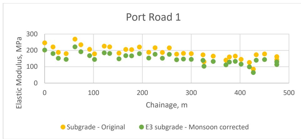
**Figure 5-19 Elastic Modulus Layer 3 Subgrade Layer Seasonal corrected at port road 1**
