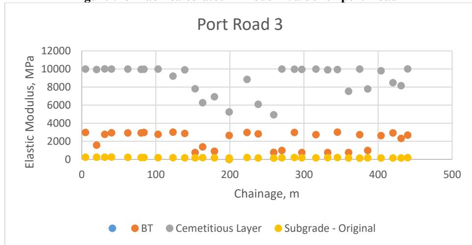
**Figure 5-9 Back-calculated E-moduli Value for port Road 3**
