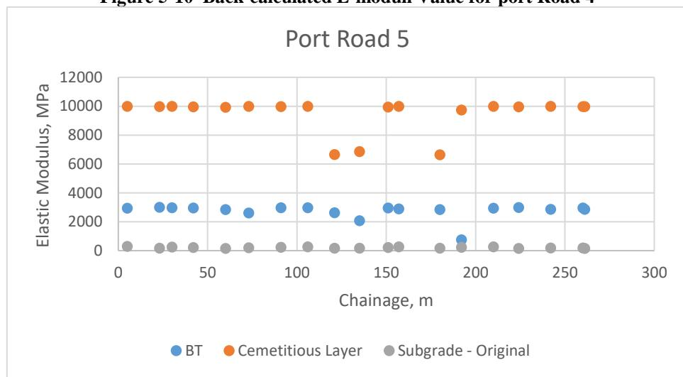
**Figure 5-11 Back-calculated E-moduli Value for port Road 5**
