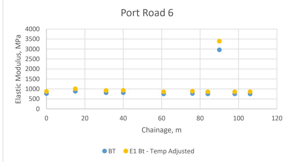
**Figure 5-18 Elastic Modulus Layer 1 Temperature Adjusted @ Port Road 6**
