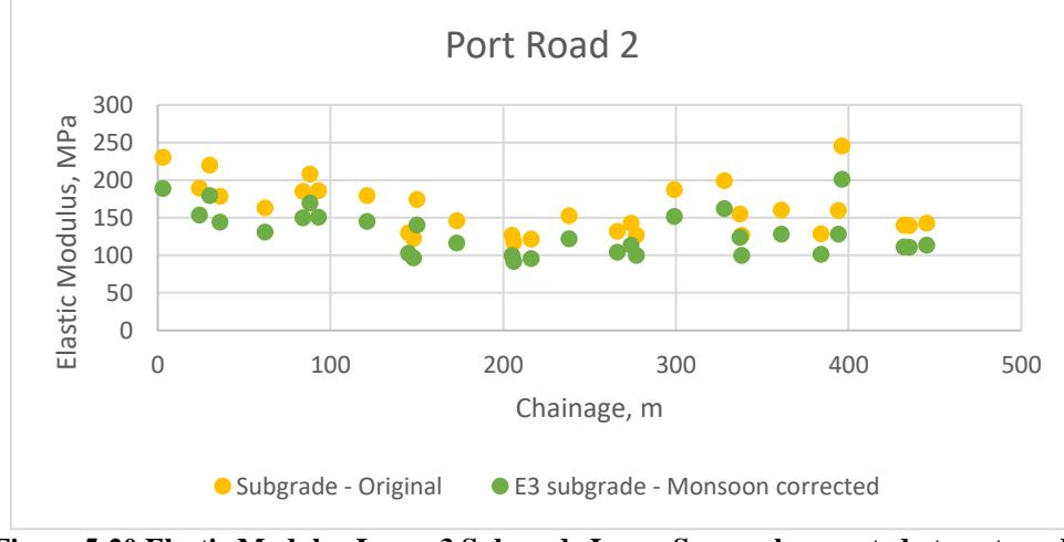
**Figure 5-20 Elastic Modulus Layer 3 Subgrade Layer Seasonal corrected at port road 2**
