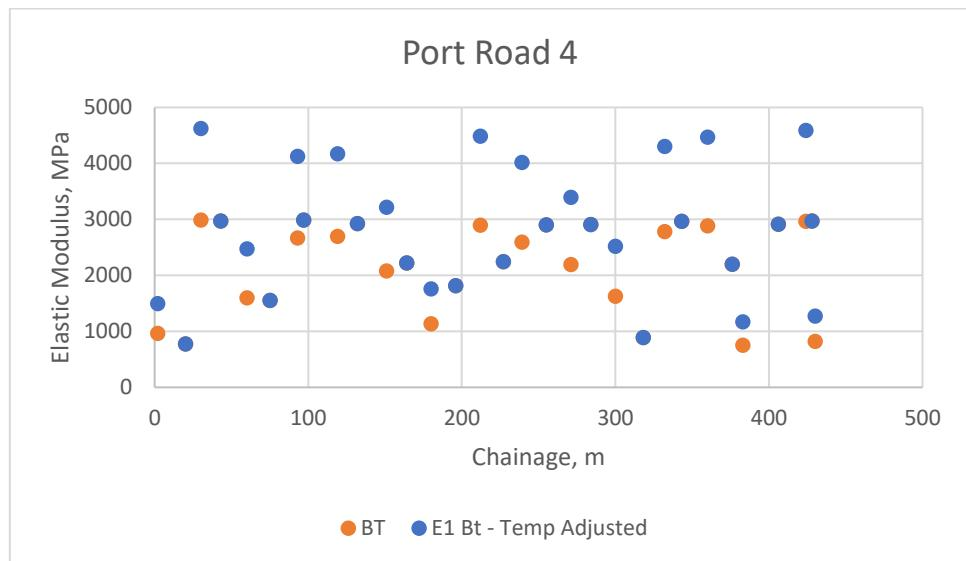
**Figure 5-16 Elastic Modulus Layer 1 Temperature Adjusted @ Port Road 4**
