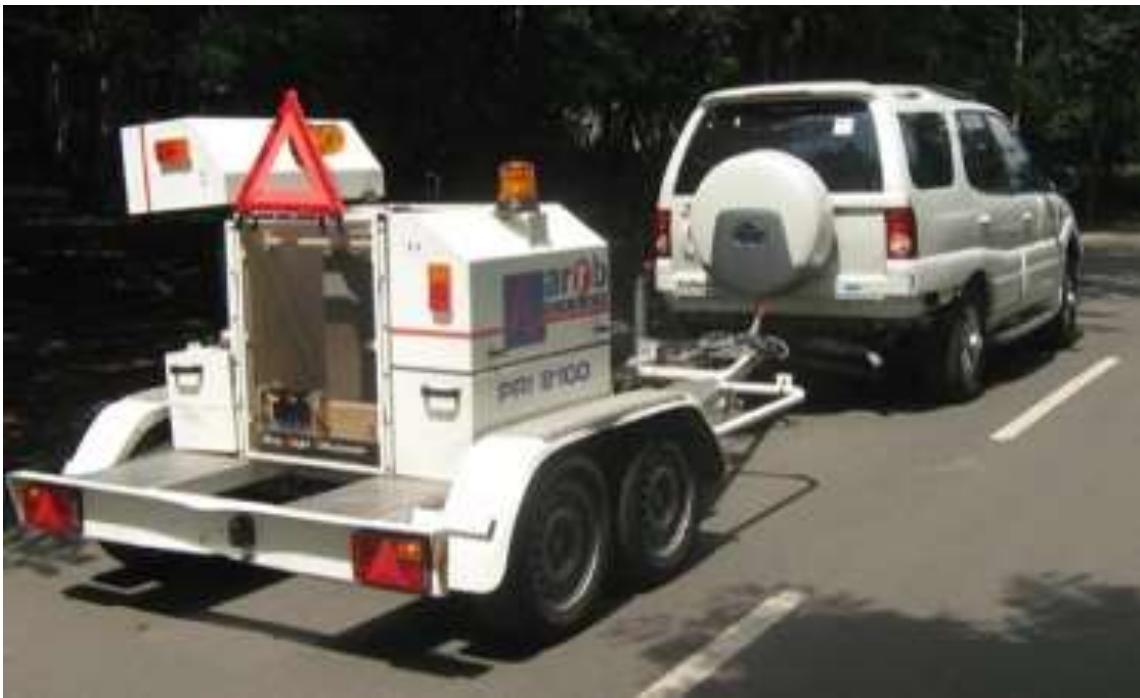
**Figure 2-2 - IRSM's Falling Weight Deflectometer – PRI2100**
