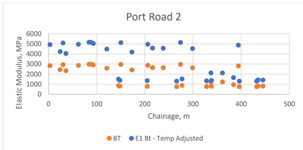
Figure 5-14 Elastic Modulus Layer 1 Temperature Adjusted @ Port Road 2
