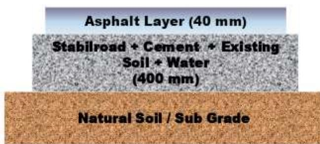
During Analysis, the same pavement thickness has been considered as 40mm Bituminous layer and 400mm Cementitious layer.
