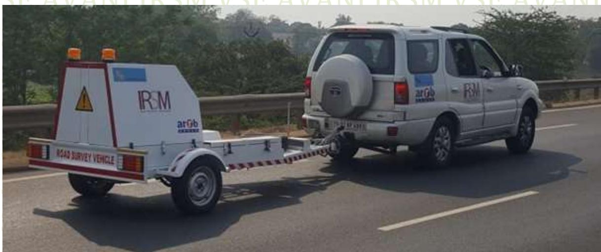
Using IRSM ERAY 20MT Falling Weight Deflectometer
