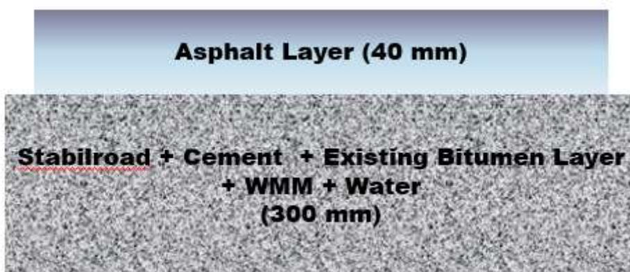
During Analysis, the same pavement thickness has been considered as 40mm Bituminous layer and 300mm Cementitious layer.
