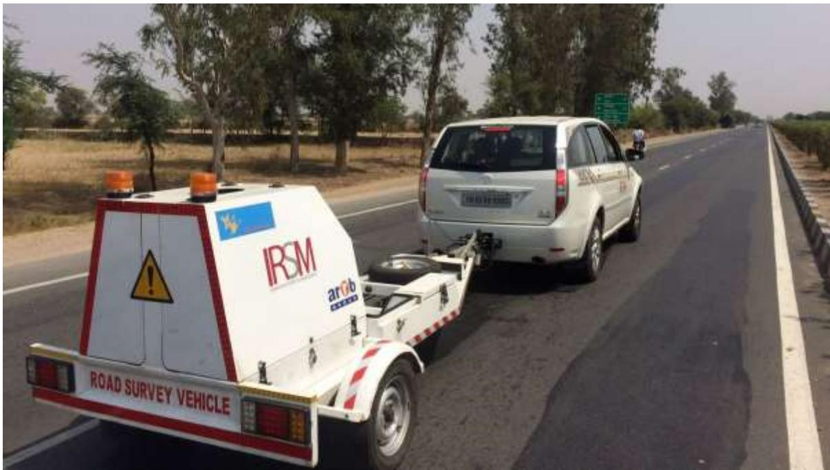
**Figure 2-2 - IRSM's Falling Weight Deflectometer – PRI2100**
