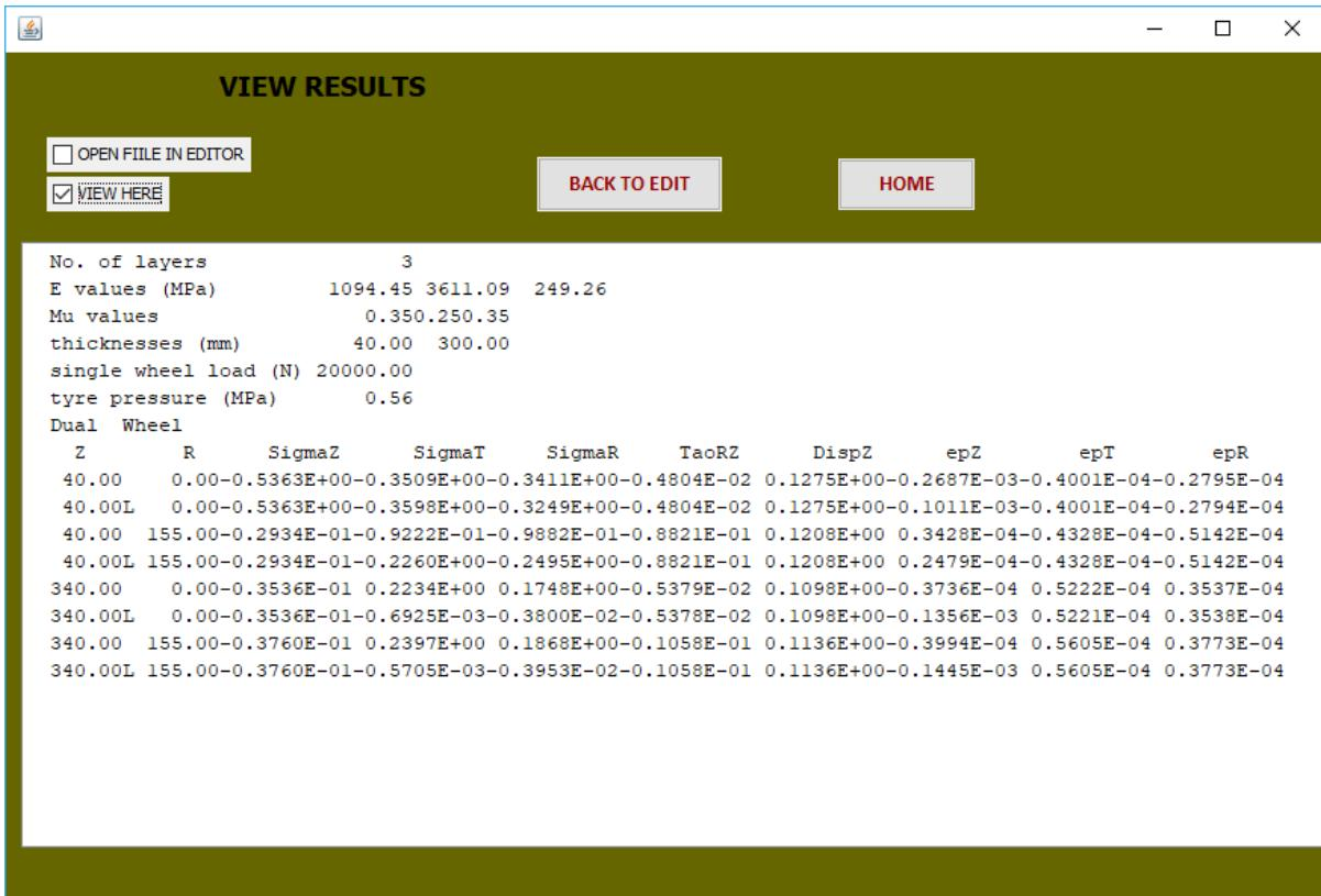
Figure 4-6 - Obtaining required strain values for checking Fatigue and Rutting performances.
