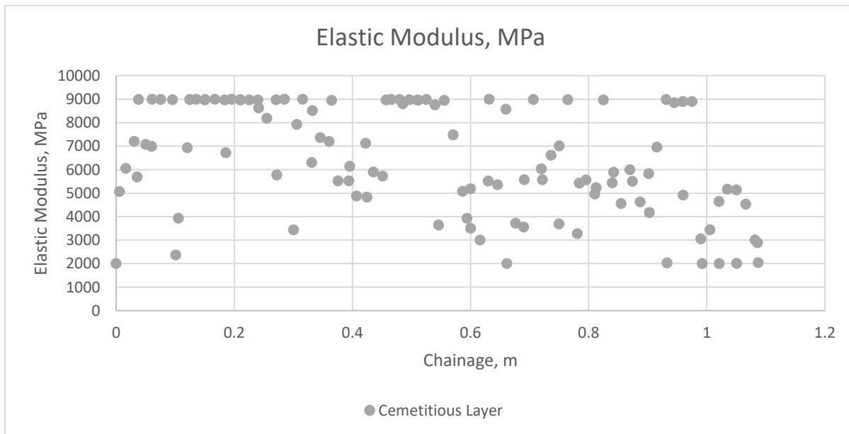
**Figure 5-4 Elastic Modulus Layer 2 Cementitious Layer**
