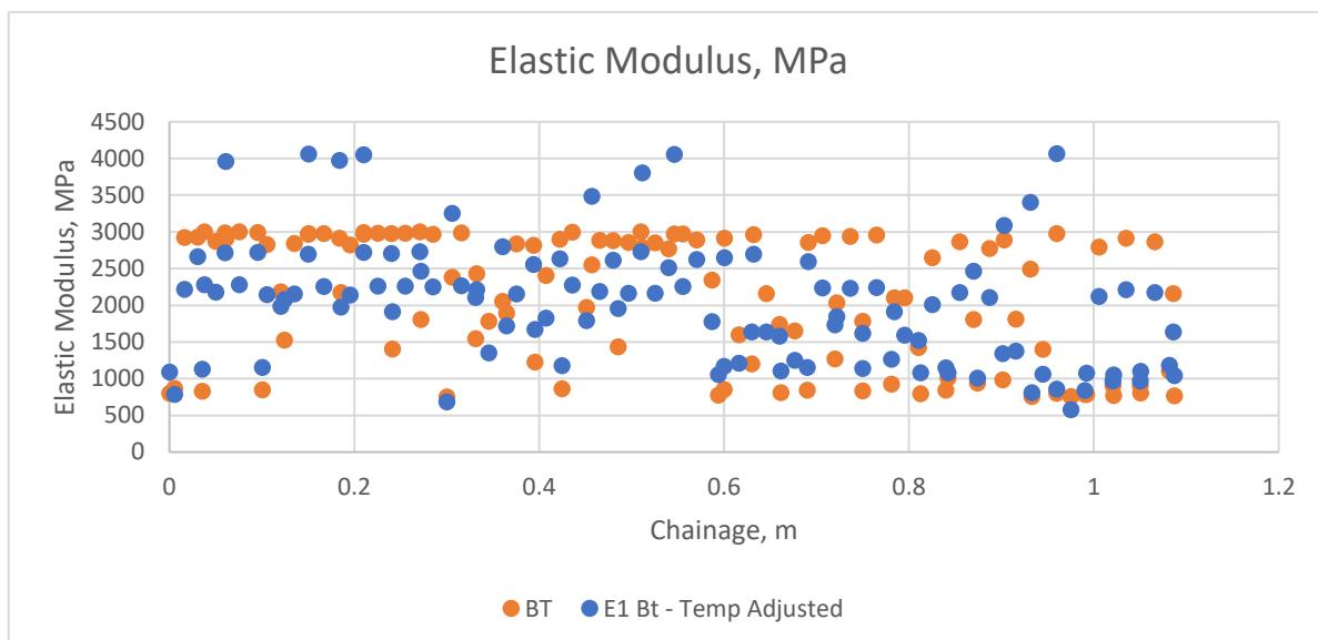
**Figure 5-3 Elastic Modulus Layer 1 Temperature Adjusted**
