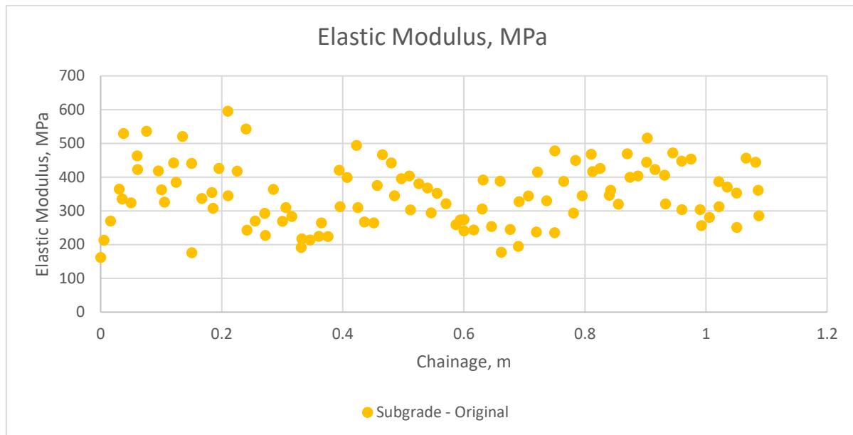
**Figure 5-5 Elastic Modulus Layer 3 Subgrade**
