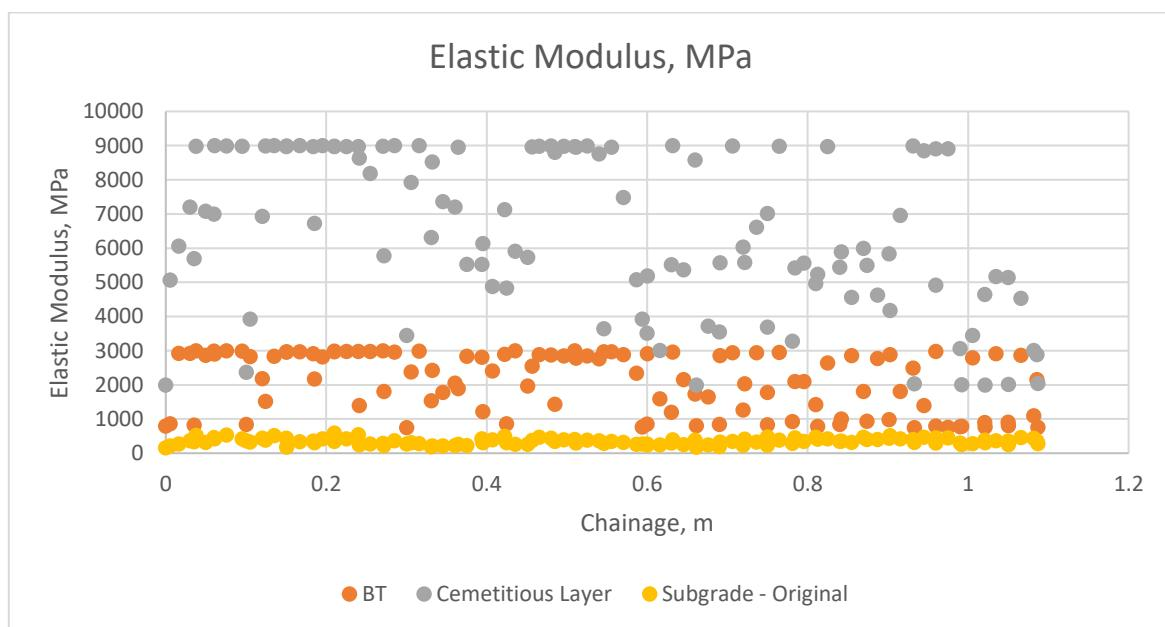
**Figure 5-2 Back-calculated E-moduli Value for NTR Marg, Hyderabad**
